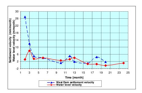
Figure 7. Velocity of the crest settlement of West Dam during filling up a reservoir
