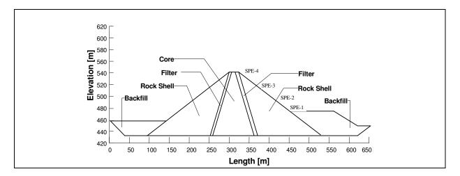
Figure 1. Schematic cross-section of the West Dam
