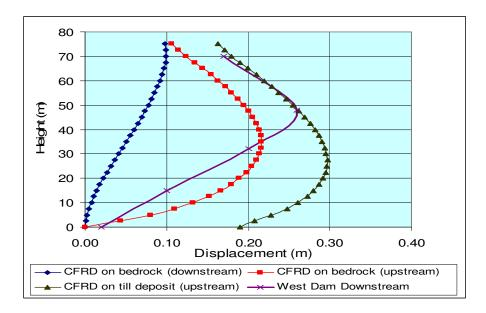
Figure 5. Total displacements of CFRD and West Dam at the end of filling up a reservoir
