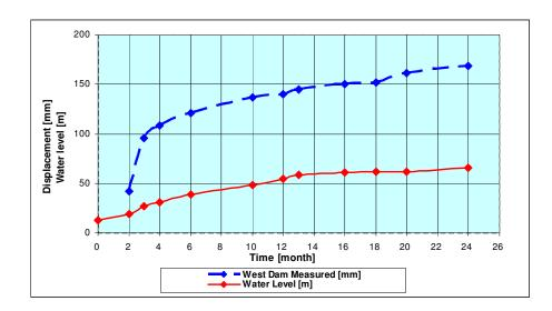
Figure 6. Settlement of the crest of theWest Dam during filling up a reservoir as a function of time
