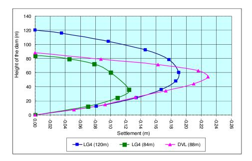
Figure 3. The calculated settlements at the end of construction of DVL and LGC dams
