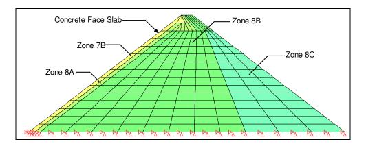
Figure 2. CFRD of 75 m of height resting on bed rock
