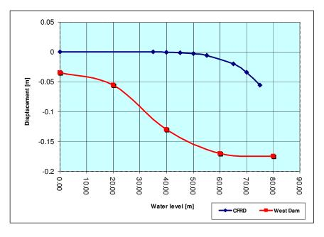
Figure 4. Settlement of crest during filing up a reservoir
